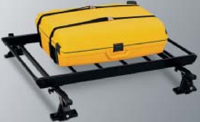
Luggage carrier, black-coated steel With adjustable ends to provide a flat surface for long loads. Dimensions: 75 x 100 cm. MZ535826
